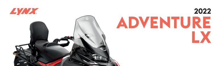
**ROTAX® ENGINE 600 ACE Engine details** Liquid-cooled, four-stroke D.O.H.C. Cylinders Displacement 600 cc Bore 74 mm 69.7 mm Stroke 7250 RPM Maximum engine speed EFI Carburation Recommended fuel type Unleaded Minimum octane 95 Fuel tank 37 liters
