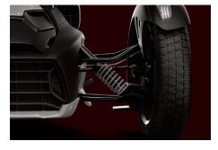
**KYB SUSPENSION** Allows 1 inch extra suspension travel and adjustability on the rear which provides four different compression settings to optimize your ride.
